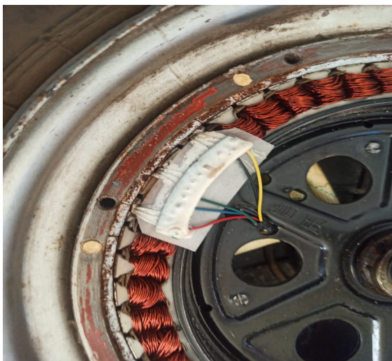
Fig. 5. Built-in Hall Effect sensor
