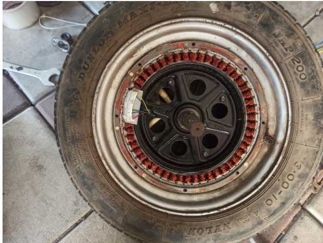
Fig. 1. Rotor and stator BLDC wheel hub motor
