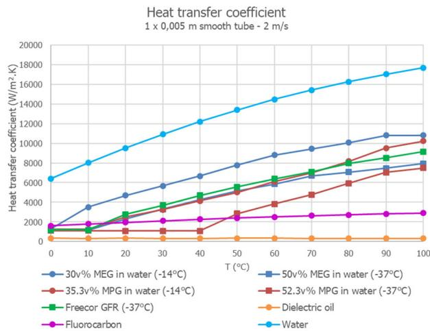
**Fig. 3.** Heat transfer coefficient of monoethyleneglycol (MEG) and monopropyleneglycol (MPG) mixtures in water compared with a Brine solution coolant (Freecor GFR-37), a fluorocarbon liquid and a standard dielectric transformer oil.
