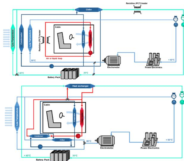
**Fig. 2.** Top: Schematic overview of a BEV thermal management system with separate battery loop, cabin loop and power electronic loop. Heat is provided by PTC heating elements. The system is coupled with the HVAC system to have auxiliary cooling of the liquid coolant. Bottom: Schematic overview of a BEV thermal management system with integrated battery and power electronic loop (trickle valve system). Auxiliary heating and cooling is provided by a heat pump system.
