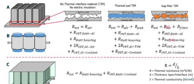
**Fig. 1.** A: Indirect water-glycol cooling of a battery pack using a bottom plate. Thermal resistance terms indicative of potential gains using TIM. B: Indirect water-glycol cooling of cylindrical cells using a cooling jacket or interleaved tube. C: Direct immersive cooling using a dielectric fluid reduces interfacial thermal resistance.
