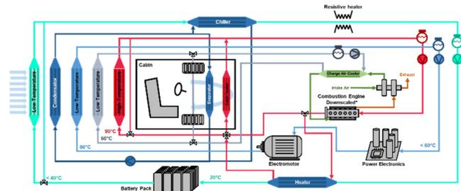
**Fig. 6.** Schematic overview of a HEV/PHEV thermal management system. In a REEV the combustion engine is downscaled.
