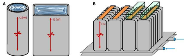
**Fig. 5.** A: Depiction of the Li-ion jelly roll inside a cylindrical and a prismatic (or pouch) cell. Heat transfer ( $Q$ ) is generally favored in axial direction. B: Combination of bottom-plate water-glycol cooling and dielectric battery tab cooling.
