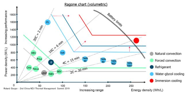
**Fig. 4.** Ragone chart comparing cooling technologies in commercial vehicles indicating apparent and projected boundaries for charge acceptance. (Adapted from Roland Berger - 2<sup>nd</sup> China NEV Thermal Management Summit 2019)
