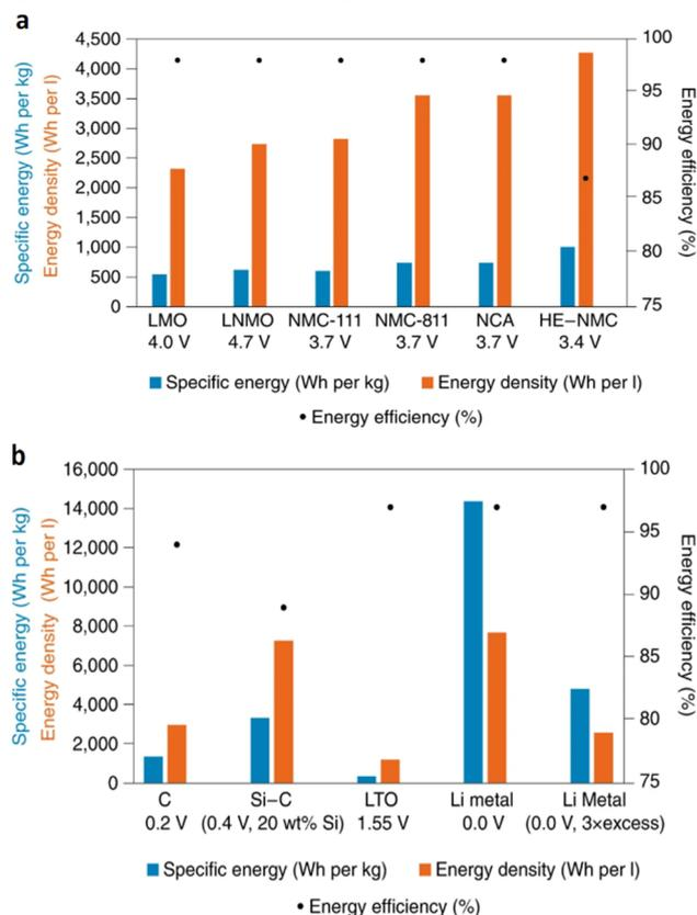
**Fig. 8.** Specific energies, energy densities, and average energy efficiencies of cathodes (a) and anodes (b) materials at materials level [Reproduced with permission from ref. 33, Copyright 2018 Springer Nature]
