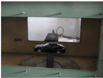
Fig. 3. The Car body with the Airfoil attached in the wind tunnel test.
