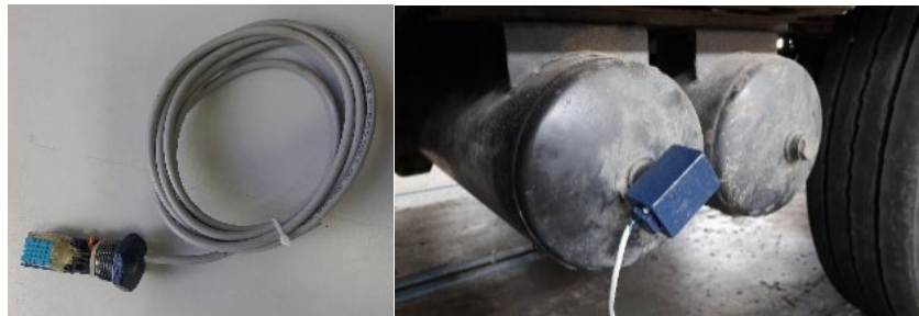
Fig. 9. Humidity sensor and mounting image.
