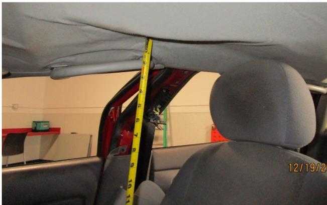
**Fig. 10.** Roof deformation pattern above the occupant's head.
