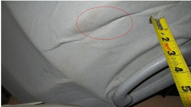
**Fig. 9.** Hair deposit on the interior roof substrate above occupant's head.
