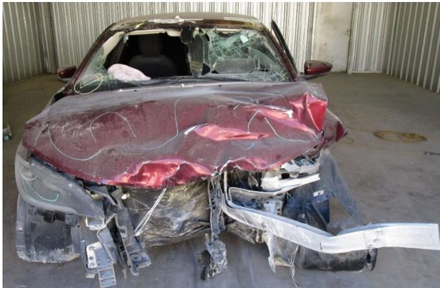
**Fig. 4.** Exterior damage pattern on the vehicle.
